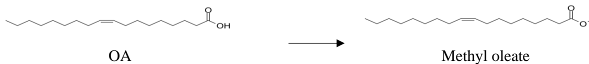
Figure 7: Structure for conversion of OA to methyl oleate.
