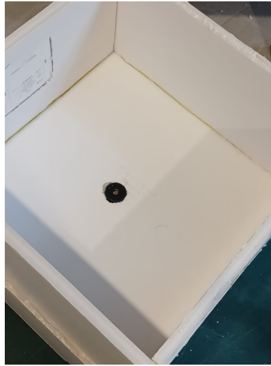
Figure 3-41 The main chamber walls glued onto the base.
