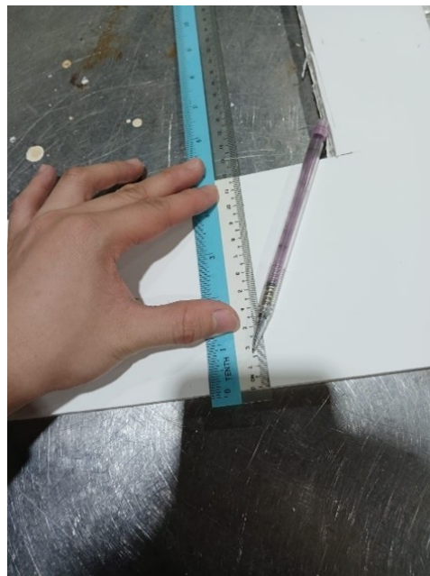
Figure 3-20 Marking one of the PVC foam boards with dimensions using a pencil and ruler.
