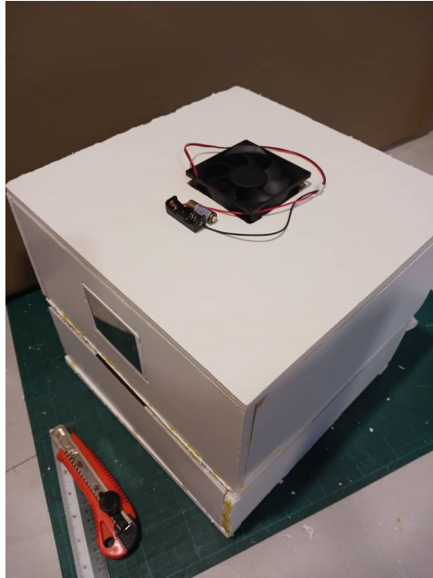
Figure 3-46 The fully assembled humidity chamber.
