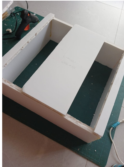
Figure 3-34 Chamber base and support glued to the bottom.
