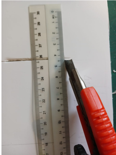
Figure 3-39 The outline being cut with a box cutter.
