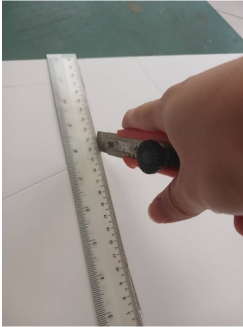
Figure 3-22 Cutting the board with a box cutter, guided by a ruler to maintain straight lines.
