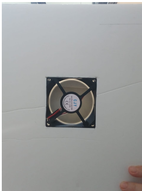
Figure 3-45 The computer fan placed into position and tested.
