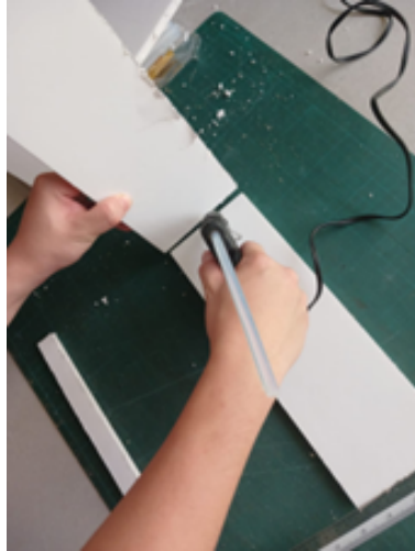
Figure 3-26 Glue gun being used to glue two board pieces together.
